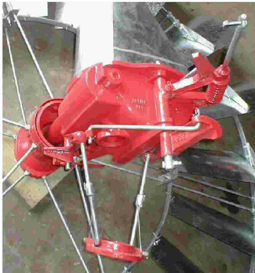
Figure 22: Buffer Device in place / Tail bone casting in place
